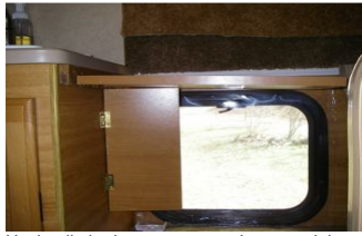
Having limited counter space I removed the shelf that would go between the sink and fridge and installed a drop down shelf.
