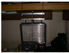
Wave 3 heater which is plumbed off the main tanks. The hanger is movable from different shelves and gets the heat off the floor.
