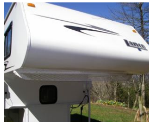
An air dam was added under the cabover.
