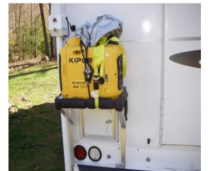
Carrier for the generator.
