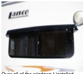
Over all of the windows I installed Vent covers. This one was designed for a Chev truck.
