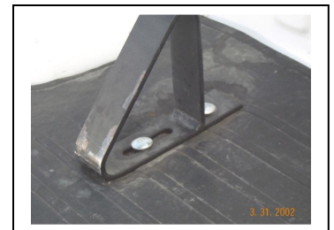
This is the bolt through method for the bedmat
